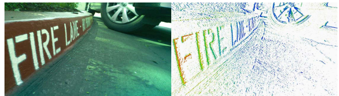
Fig. 15. Captured color image and corresponding signal phase/distance (close objects are reddish and distant objects are bluish).
