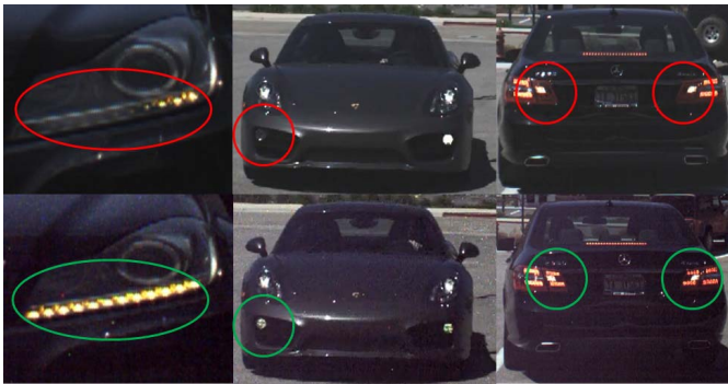
Fig. 9. Flickering LED turn lights, headlights, and brake lights image captures three-exposure HDR (top) versus pLFM HDR (bottom).
