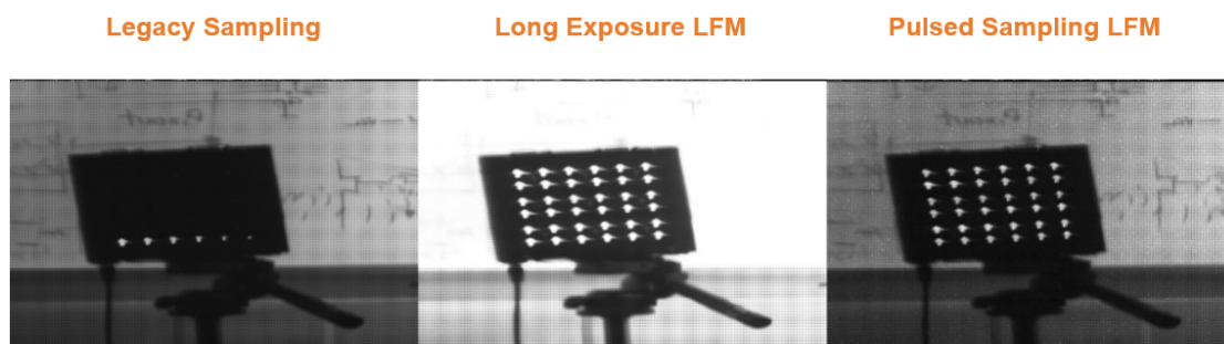
Figure 1. LFM Samplings at 30 fps 10% Duty Cycle 10 ms Period (100 Hz)
