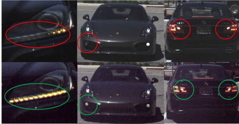
Figure 5. Multi-exposure HDR (top) vs. LFM HDR (bottom) Image Captures of Flickering LED Lights
